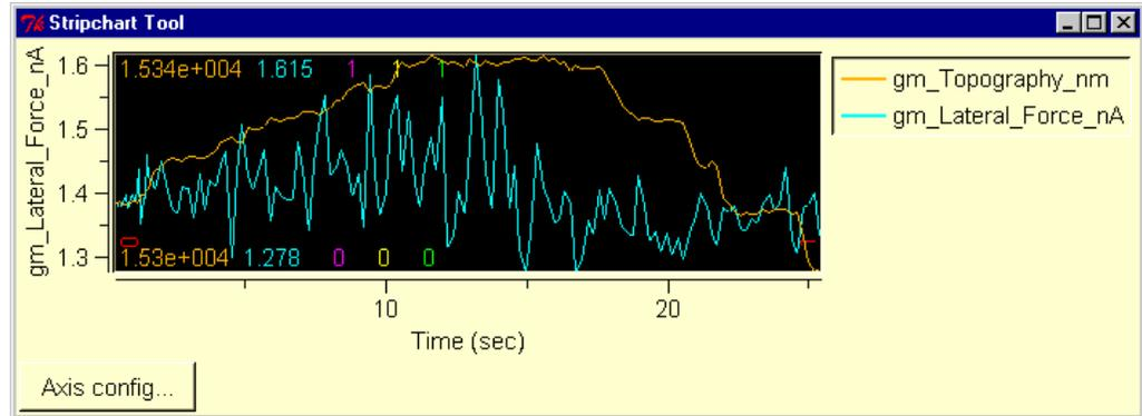
By default, the Strip chart shows both Topography and Lateral Force as a function of the arc-length of the modification so far. You can choose to graph data versus time, versus arc length in nanometers, or versus the X or Y coordinate where the data was collected.
