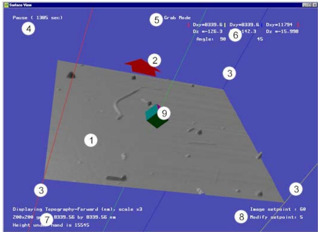
1. Surface – 3D Display of the height information from the plane specified by the Height Plane control.
